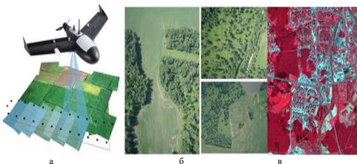
Figure 3 - Monitoring of the Earth's surface from the UAV: a - the moment of the survey; b - optical image of the area in the visible wavelength range; c - spectral image of the area
