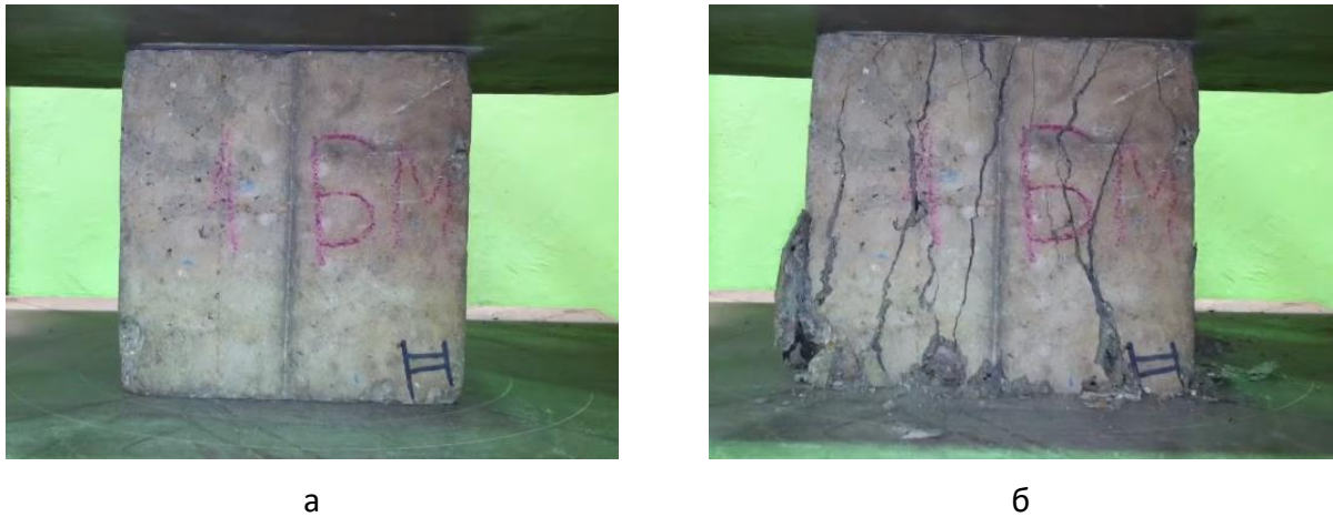
Figure 5 - Testing of concrete samples (cubes) for compressive strength [2]: a – cube before the test, b – cube after the test
