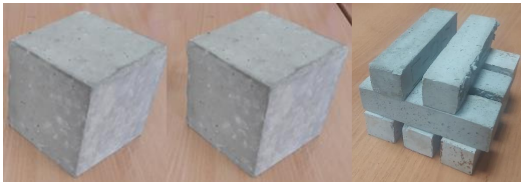
Figure 3 - Ready-made samples-cubes and a batch of ready-made samples-beams (28 days)
