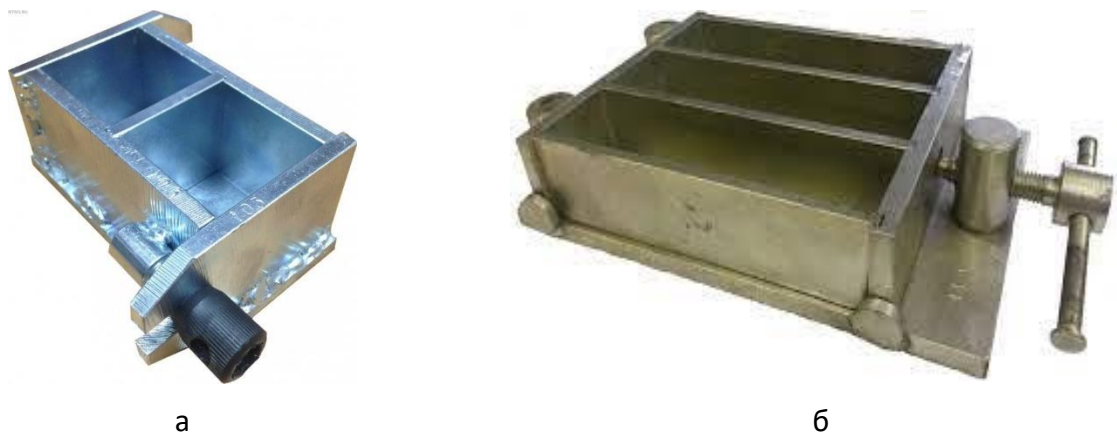
Figure 2 - Molds for the manufacture of concrete samples: a - cubes 2FK-100; b - beams 3FB-40
