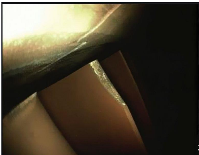
Figure 5 - Damage to the blades of the 1st stage of the turbine (erosive wear of the leading edge)
