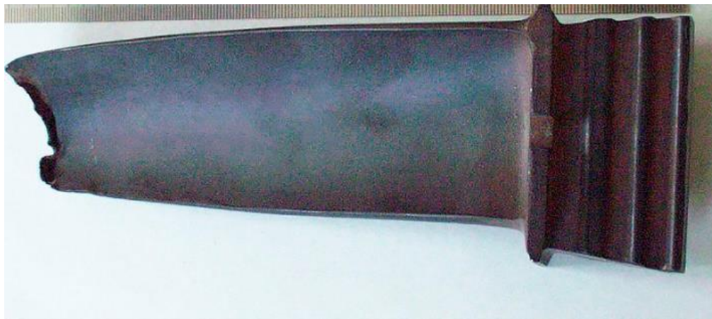
Figure 3 - Damaged turbine blade
